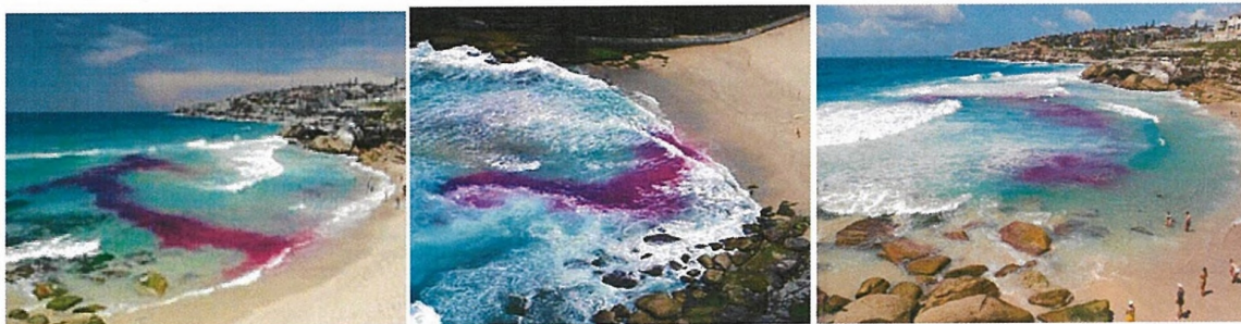
Figure 3. Examples of purple dye releases in rip currents at Tamarama Beach showing variable circulation patterns.
